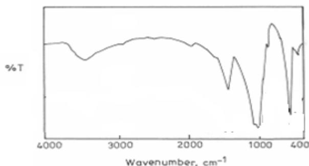
Figure 1: IR spectrum band of the prepared nano hydroxyapatite.
