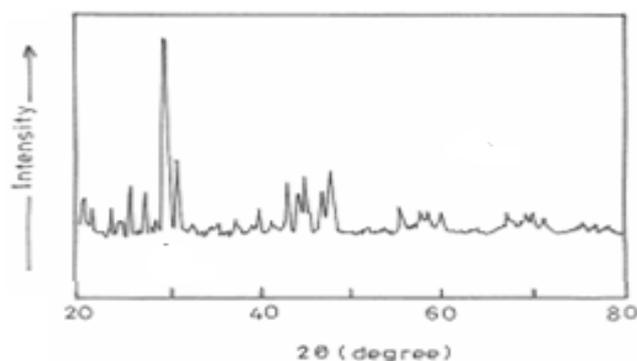
Figure 2: X-ray pattern of the prepared nano Hydroxyapatite
