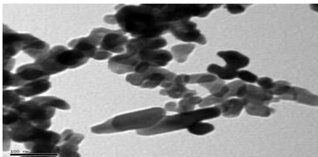
Figure 3: TEM image of the prepared nano hydroxyapatite
